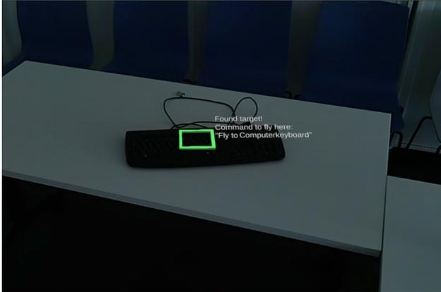
**Figure 5: Illustration of the highlighting of targets done in augmented reality. After using the command *Fly to Computerkeyboard*, the UAV approaches the target according to the calculated path.**
