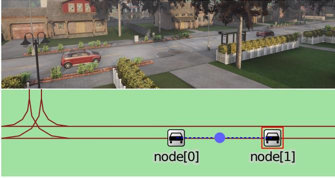
Figure 1. Sample screenshots of CARLA (top) and Veins (bottom) running in tandem to simulate two cars driving autonomously through a suburban area with buildings, hedges, and trees while exchanging information wirelessly.
